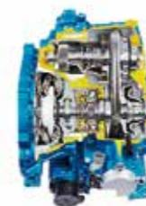
CVT(Continuously Variable Transmission(無段
